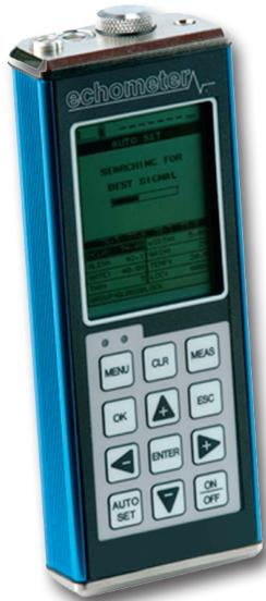
The Echometer ultrasonically measures the elongation, stress, and load in fasteners, quickly and accurately, and displays the result on an easy to read screen. The measurement is achieved by determining the change in the transit time of any ultrasonic shock wave along the length of the fastener as the fastener is tightened.
