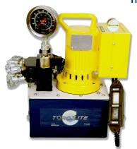
These pumps have been continually upgraded over the last 40 years and even some of the originals are still in service. Equipped with a 1½ hp, single-phase universal motor, they have a noise level of 90-95 dB(A). Offer an incredible weight-to-performance ratio for any of our electric/hydraulic pumps, and are CSA rated for intermittent duty.
