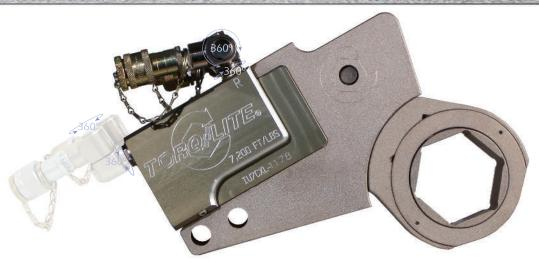
Inline ratcheting wrenches require minimum clearance while applying torque on the same plane as the nut, providing a marked improvement over square drive socket wrenches. Our patented design breakthrough reduced the overall dimensions of the inline ratcheting head allowing it to fit almost every application. Our IU-XL Series tool capacities range from 100 to 50,000 foot pounds of torque using a 10,000 p.s.i. hydraulic pump. "Extra light, dependable, and fits where others can not"
